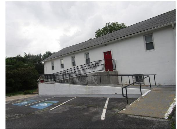
Parking spaces in the center of the lot can be replaced with pervious pavement to capture and infiltrate the stormwater runoff from the parking lot. A preliminary soil assessment suggests that the soils have suitable drainage characteristics for green infrastructure.
